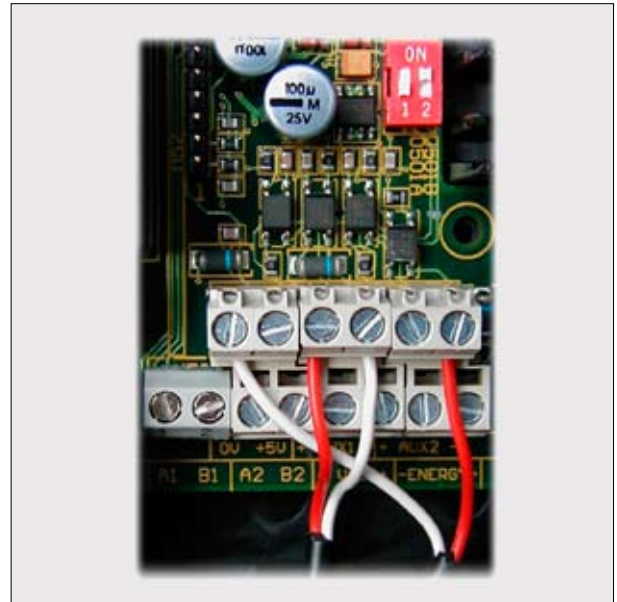
AUX1 galvanic isolated - AUX2 not isolated
